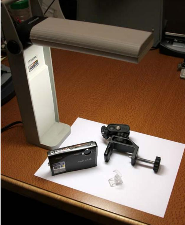
1. A Fluorescent light source. The Ott-Light Truecolor is very effective due to its small footprint, daylight color temperature, light weight and adjustability.
