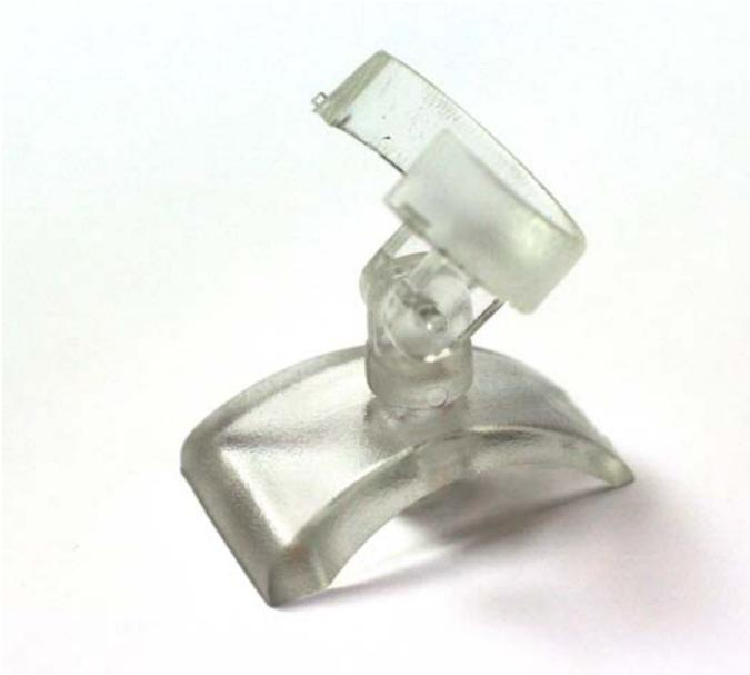
4. A device to hold the ring. The one shown allows you to adjust the angle of the ring, thereby eliminating the need to adjust the angle of the camera.
